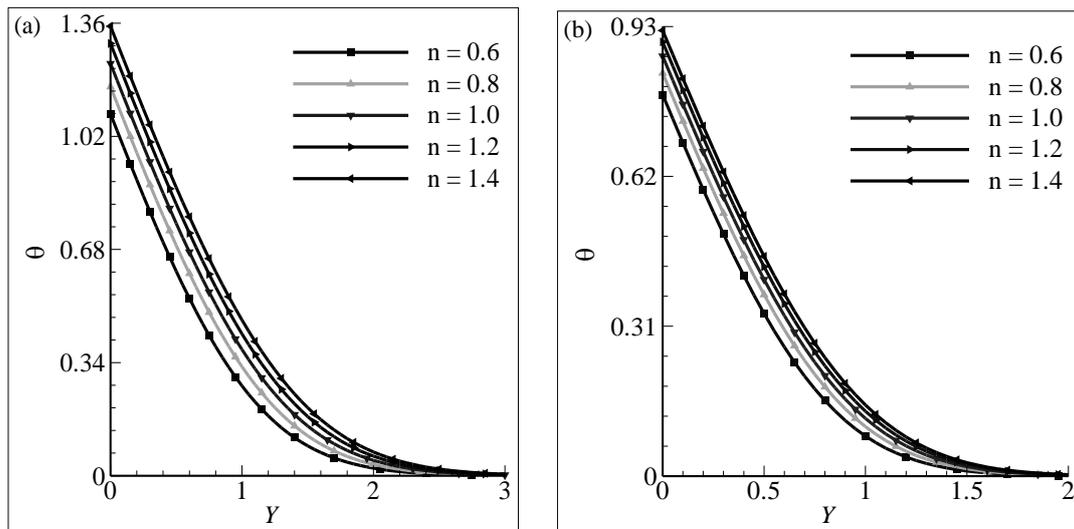
Fig. 5 Temperature distribution for different  $n$  at  $X = 2$  for (a)  $Pr = 10$  and (b)  $Pr = 50$ .
